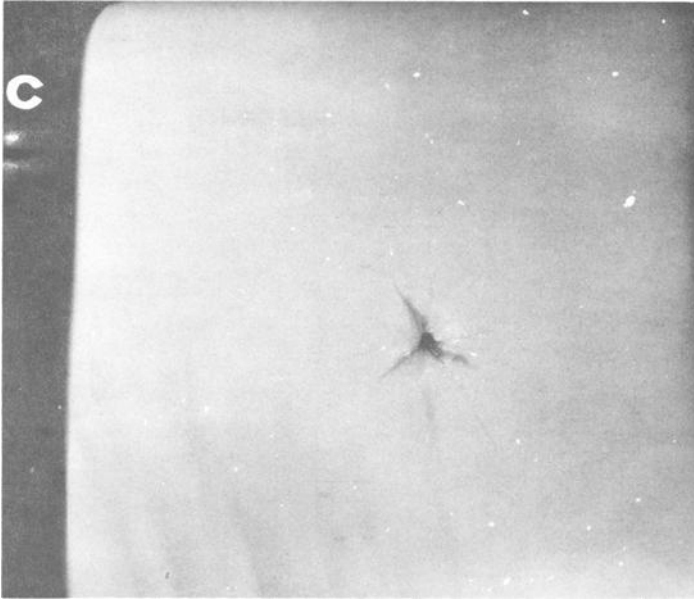
FIG. 11—Roentgenogram of face of gelatin block after Test C (AFIP Neg. 73-12619-3).
